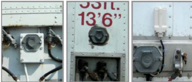
Various locations for the 7-way receptacle, photos left and center. Photo on right is an example of proper device placement.
